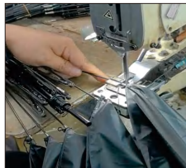
8. 露先と生地縫製 Canopy Stitched to Ribs
